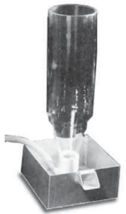
*Hatching bottle complete with tank*
