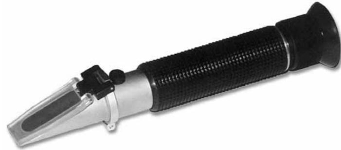
This Salinity Refractometer is for quick and easy measurement of the salinity in water. This simple to use refractometer measures in parts per thousand (ppt) or specific gravity. The meter operates with natural light and has no moving parts to wear out. Hatchery and farm tested for reliability and durability.
