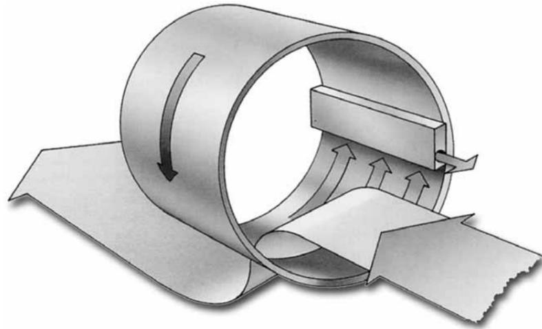
Microsieving is an efficient and reliable technique for separation of particles from all kinds of liquids. Hydrotech develops and manufactures high performance filters for water purification and product recovery.
