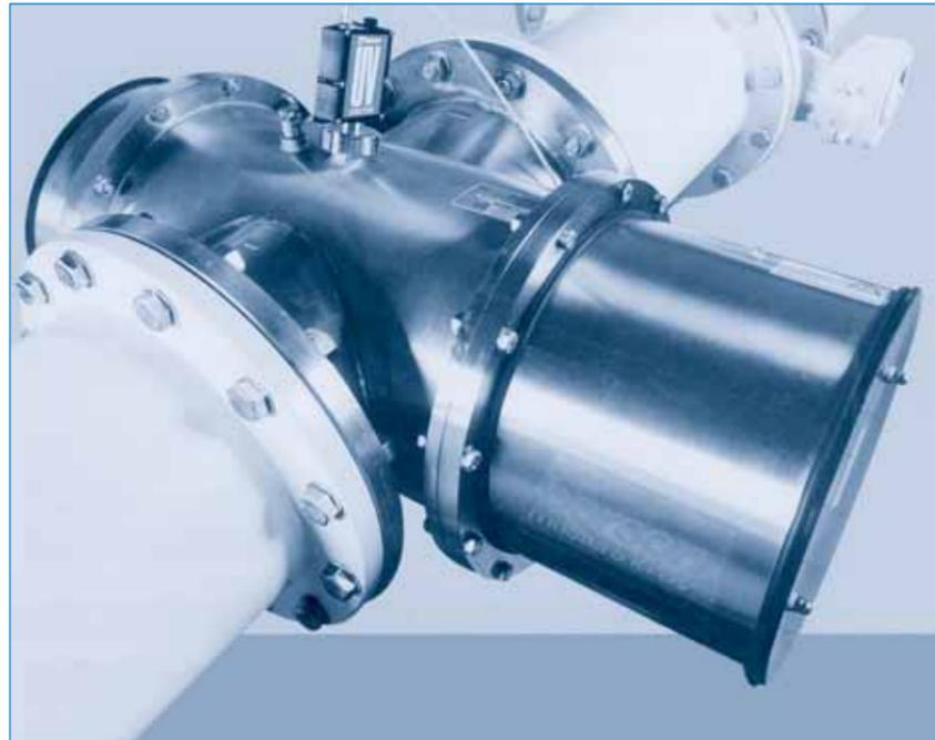
An alarm is given when the UV-dose drops below a preset level. This for example can be caused by extra pollution of the incoming water. The quartz tubes in the UV-chamber can be cleaned with a manual or automatic wiper, even when the unit is in function.
